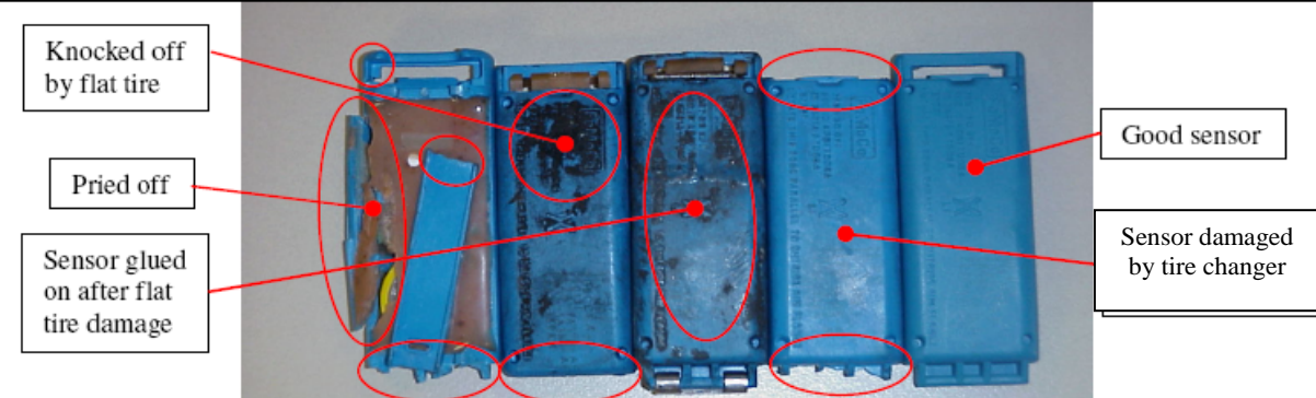
3 of the 4 sensors damaged due to improper removal or installation.
