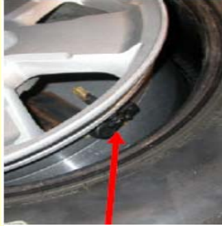
The valve mounted sensor is bolted to the valve stem
