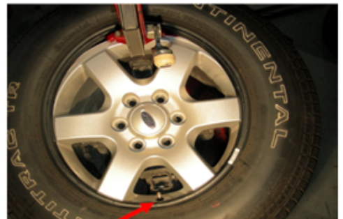
Bottom Bead Installation
