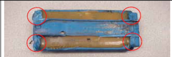
Driven on a flat tire. All four sensor feet are crushed.
