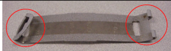
Cradle damaged from driving on flat tire.
