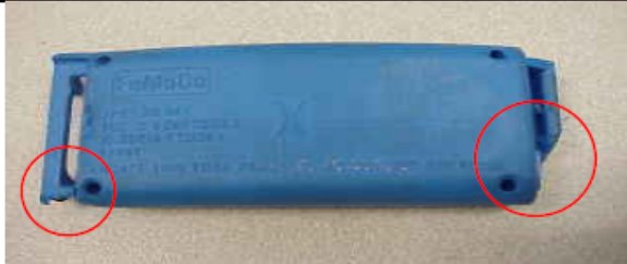
Broken CPA Retaining feature and Hinge tabs.
