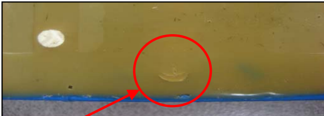
Indentations in potting from force being applied
