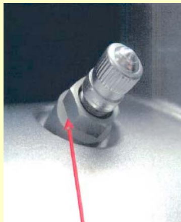
Bolt-On Stem Note: Aluminum Nut Sensor Type 1&2
