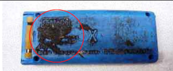
Sensor damage due to driving on flat tire for extended period. Tire material embedded in sensor.
