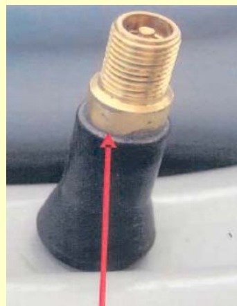
Snap-In Stem Note: Brass Collar Sensor Type 6
