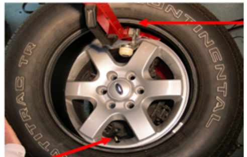
Top Bead Installation
