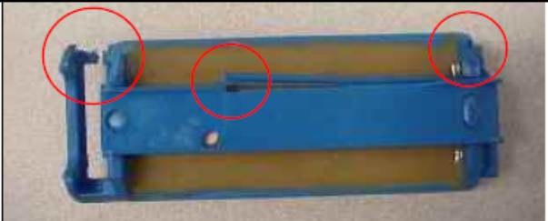
Sensor broken by Tire Changer Bead Breaker Paddle.
