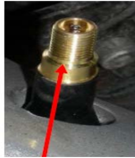
The Snap-In TPMS sensor has a brass collar
