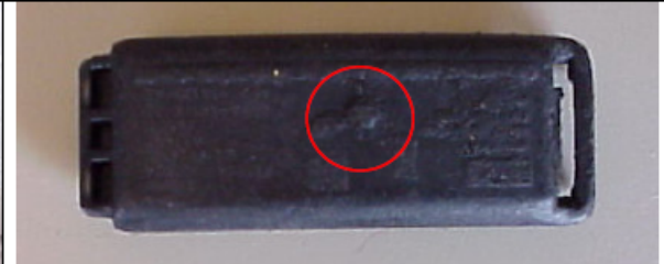
Air Intake Port plugged with tire material.
