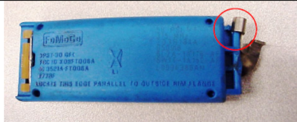
Hinge Tab torn by improper tire removal.
