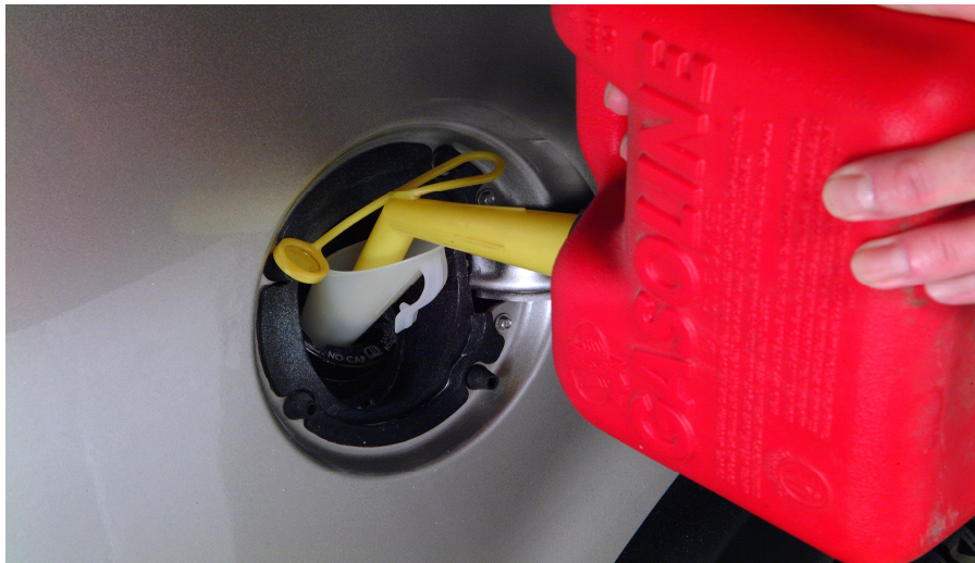
Figure 10. Adding Fuel from a Portable Container
