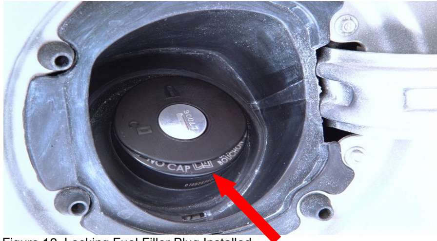
Figure 12. Locking Fuel Filler Plug Installed
